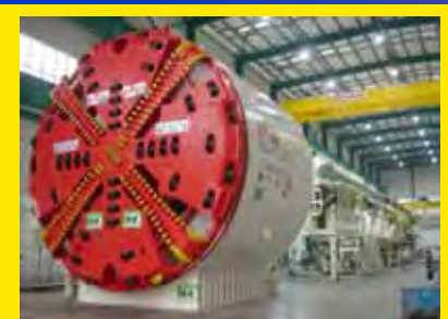
Mixed Shield TBM
