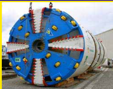
Slurry Shield TBM
